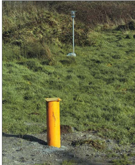
Wellhead of borehole used to monitor groundwater level and water quality, and Bergerhoff gauge used to monitor dust levels, adjacent to TMF at Gortmore
