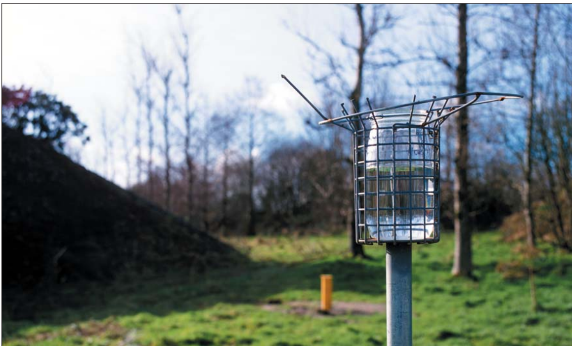
Bergerhoff gauge used to measure the concentration of lead in deposited dust
