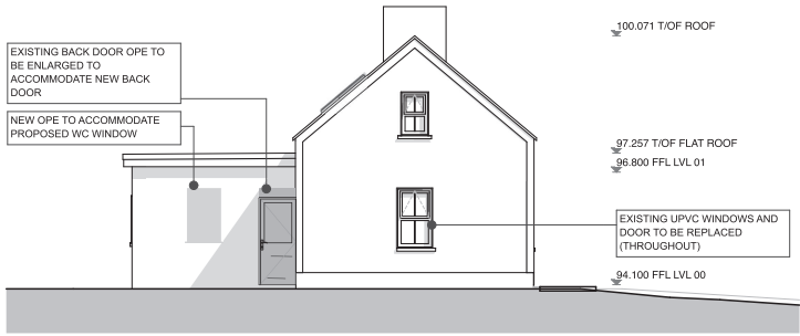
NORTH ELEVATION - EXISTING 1:100
