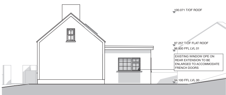
SOUTH ELEVATION (REAR) - EXISTING 1:100
