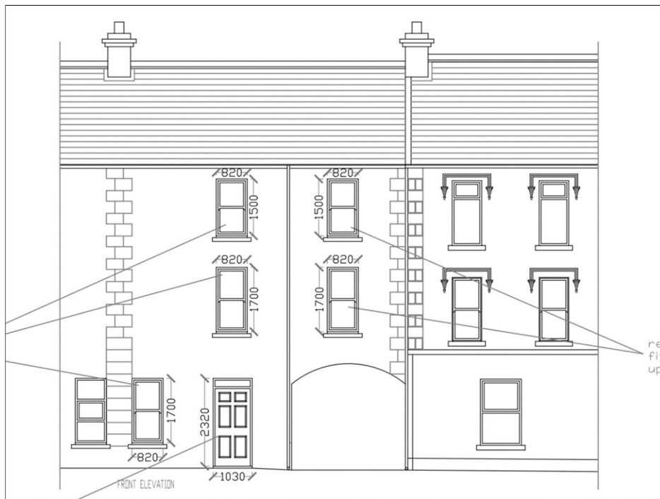
Figure 3: Proposal drawing for Main Street elevation of subject building received with further information on 10 th February 2025
